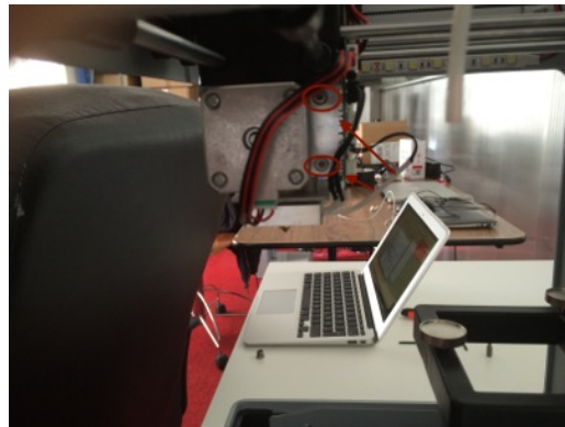
21. Remove block screws (right)
