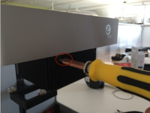
12. Remove 2 screws from front
