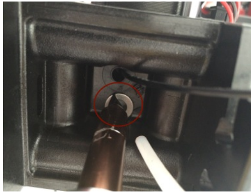
17. Unscrew and remove head nut
