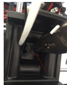
15. Remove housing retainer
