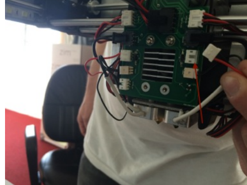
13. Remove 2 fan connector as shown on picture
