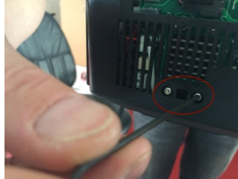
11. Remove 2 screws on the back of the cover
