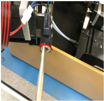
6. Screw the new teflon retainer using a 11 mm wrench
