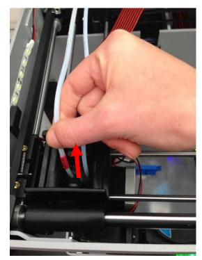
5. Remove the Filament housing retainer
