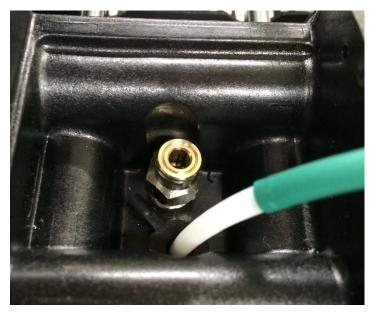
8. Insert back the teflon tube. The teflon tube must be inserted 27.5 mm deep.
